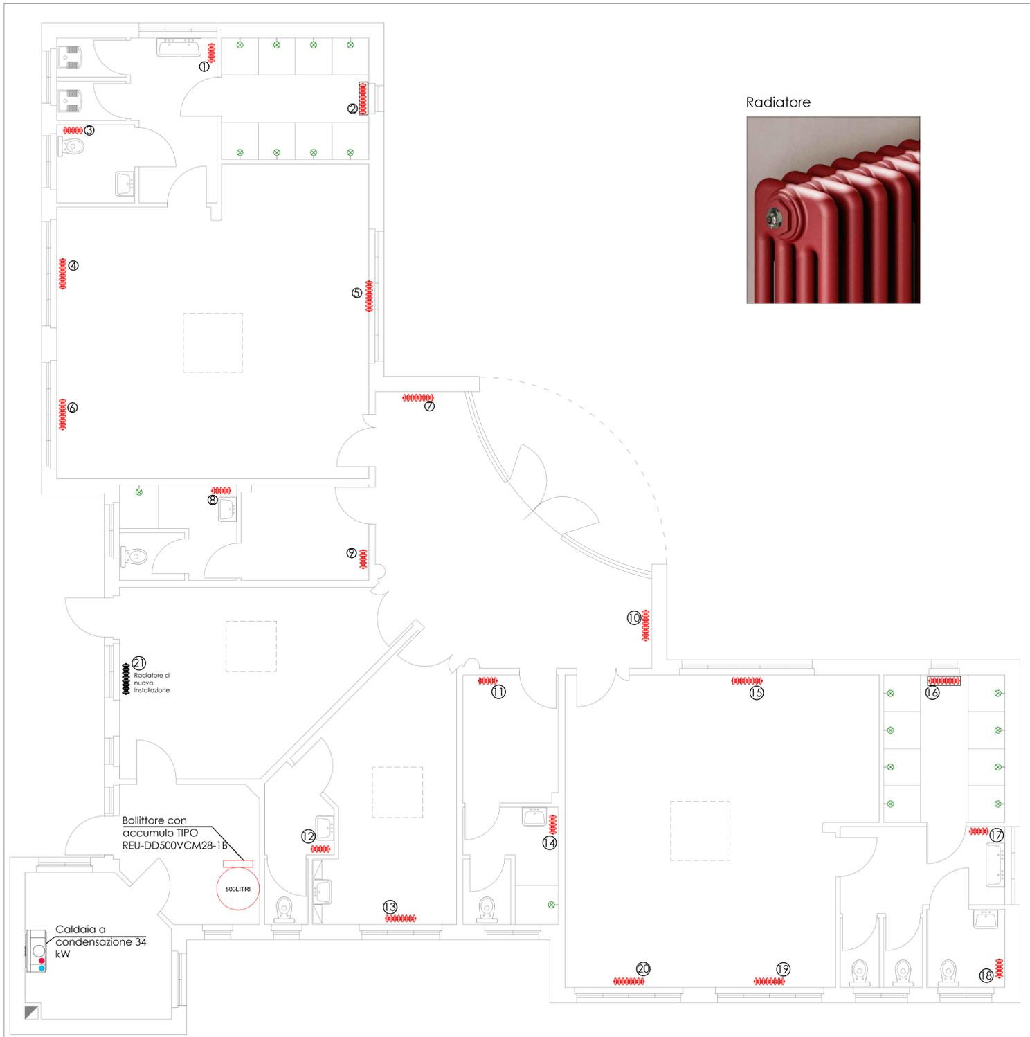
PIANTA IMPIANTI TERMICI ED IDROSANITARI PIANO TERRA
